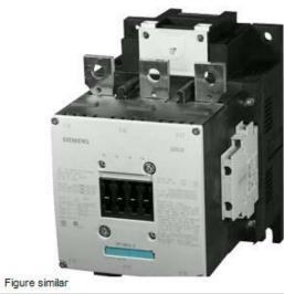
CONTACTOR, 160KW/400V/AC-3 AC(40...60HZ)/DC OPERATION UC 110-127V AUXILIARY CONTACTS 2NO+2NC 3-POLE, SIZE S10 BAR CONNECTIONS CONVENT. OPERATING MECHANISM SCREW TERMINAL
